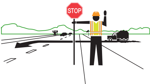
Figure 10 Flagging for trucks turning left or crossing highway
