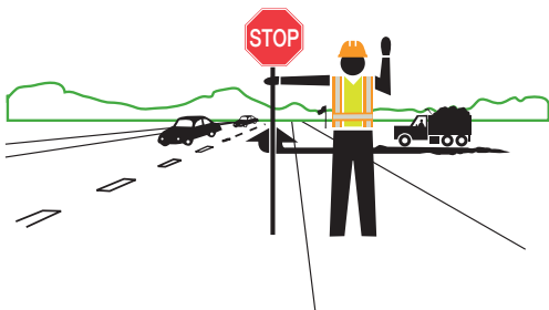
Figure 9 Flagging for right-turning trucks at haul road
