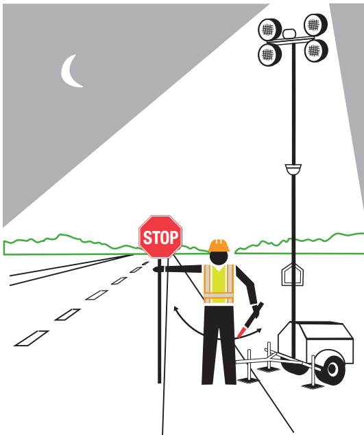
Figure 13 Flagging to stop traffic at night
