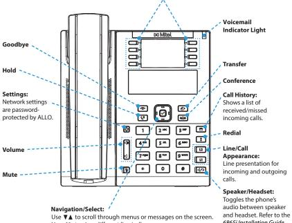
Use **◄** ► to view different line/call appearances. character on the left, and pressing the ▶ key sets the option. Alternatively, pressing the center key sets the option as well on specific screens.
